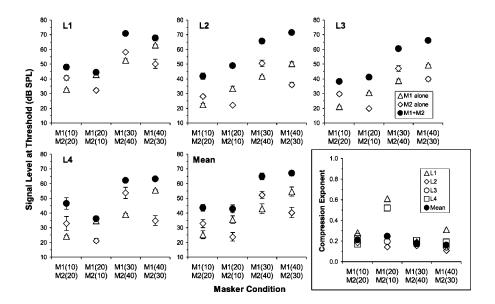
FIG. 1. The results of Phase 2 of the experiment, showing signal thresholds in the presence of the single (open symbols) and combined (closed symbols) maskers. Error bars show standard errors. The lower right panel shows compression exponents derived from the data (see the text for details).
